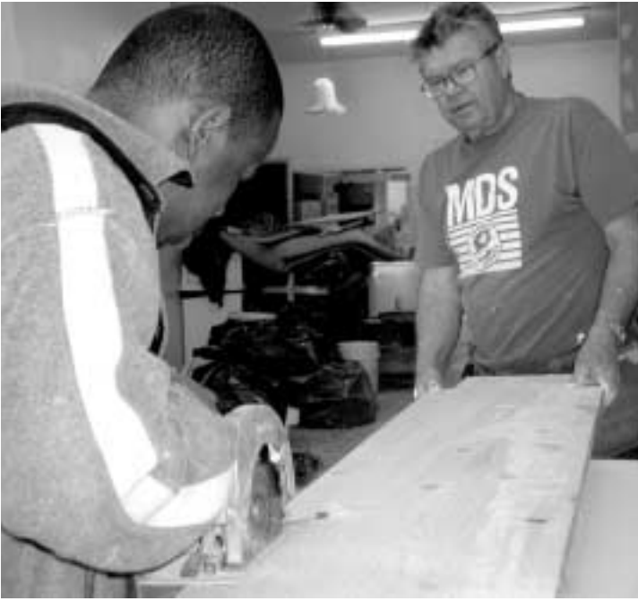
Volunteer Jose Henriquez rips a shelf board with a circular saw while Bernard Martin steadies the end and coaches the process.
